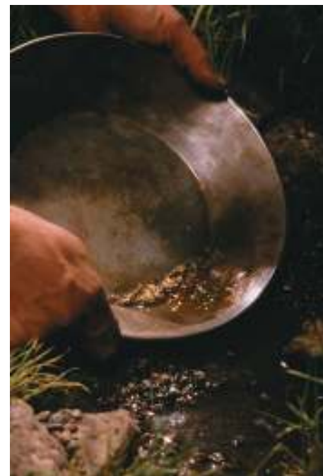
▲ In panning for gold, prospectors use density differences to separate gold from the gangue.
