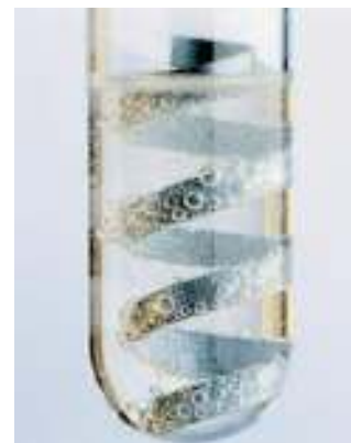
▲ Zinc metal reacts with aqueous hydrochloric acid to give hydrogen gas and aqueous \text{Zn}^{2+} ions.
