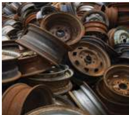
The rusting of these wheel rims is a slow but spontaneous reaction.
