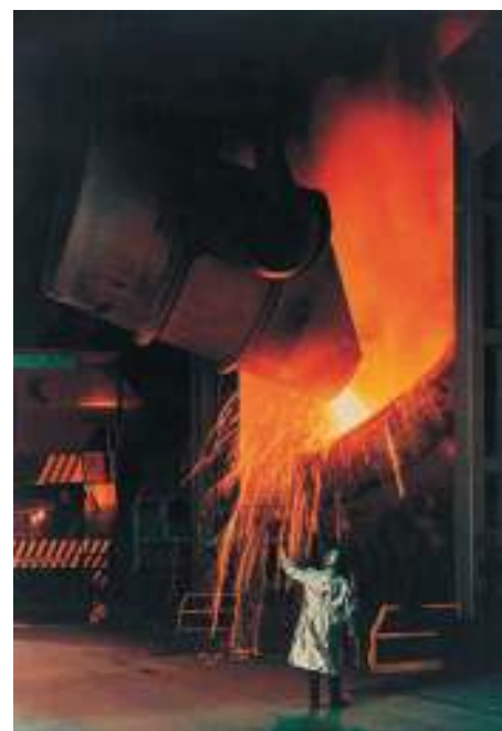
▲ Using the basic oxygen process to make steel.
