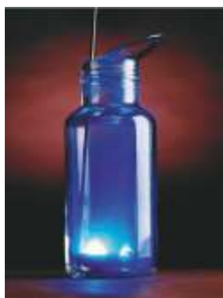
Hot, molten sulfur burns in oxygen with a blue flame, forming gaseous sulfur dioxide, SO 2 .
