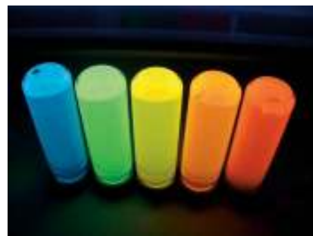
▲ The color of these semiconductor nanoparticles, called quantum dots, varies from red to violet as the size of the nanoparticles decreases.
