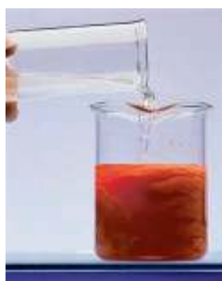
The solutions are mixed to give solid HgI 2 , which is removed by filtration.
