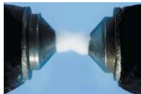
Figure 7.16 Paramagnetism. Why does liquid O_2 stick to the poles of a magnet?
