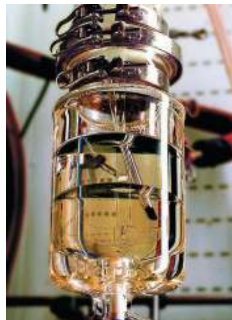
▲ As surprising as it sounds, the bottom liquid in this reactor is composed of ions.
