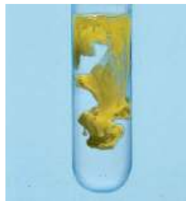
▲ Reaction of aqueous \text{Pb}(\text{NO}_3)_2 with aqueous \text{KI} gives a yellow precipitate of \text{PbI}_2 .
