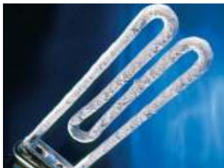
▲ Boiler scale, consisting of insoluble metal carbonates, such as CaCO 3 and MgCO 3 , forms when hard water is heated.
