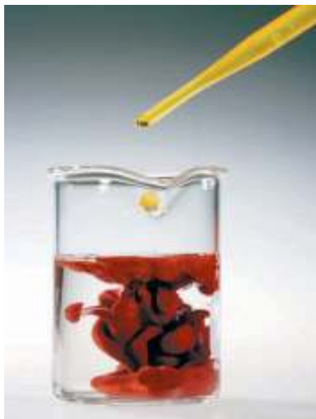
▲ Addition of aqueous K_2CrO_4 to aqueous AgNO_3 gives a red precipitate of Ag_2CrO_4 and a saturated solution of Ag_2CrO_4 .
