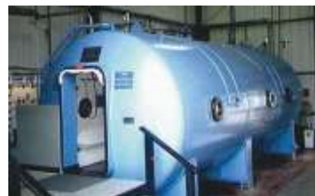
▲ Divers who ascend too quickly can develop the bends, a condition caused by the formation of nitrogen bubbles in the blood. Treatment involves placing the diver into this decompression chamber and slowly changing the pressure.
