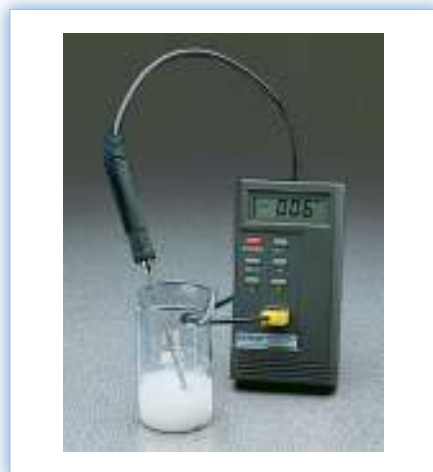
Figure 8.6 The endothermic reaction of barium hydroxide octahydrate with ammonium chloride. The reaction draws so much heat from the surroundings that the temperature falls below 0 °C.
