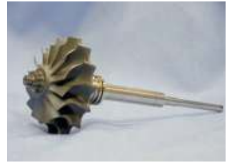
▲ A silicon nitride rotor for use in gas-turbine engines.
