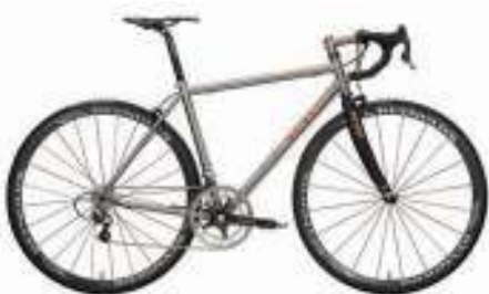
▲ This titanium bicycle doesn't corrode because of a hard, impenetrable layer of \text{TiO}_2 that adheres to the surface and protects the metal from further oxidation.
