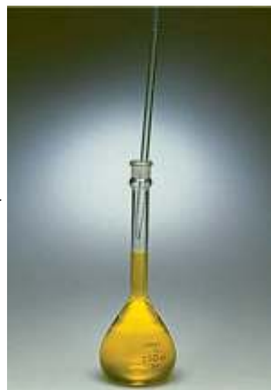
Further solvent is added to reach the calibration mark on the neck of the flask, and the solution is shaken until uniform.
