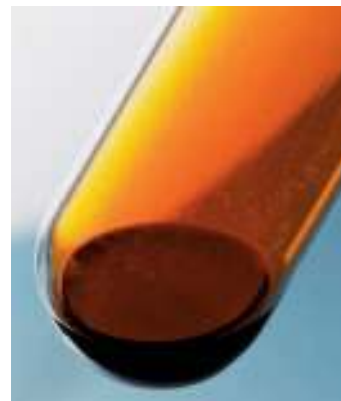
▲ In a closed container, liquid bromine and its vapor are in a dynamic equilibrium.
