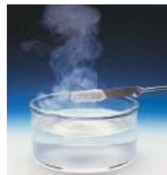
▲ The reaction of P_4O_{10} with water produces enough heat to convert some of the water to steam.
