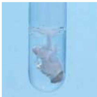
▲ Reaction of aqueous \text{AgNO}_3 with aqueous \text{Na}_2\text{CO}_3 gives a white precipitate of \text{Ag}_2\text{CO}_3 .
