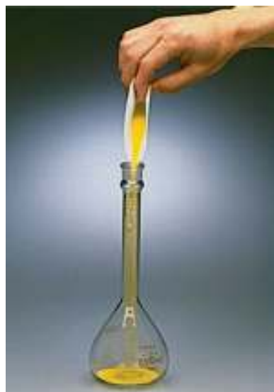
A measured number of moles of solute is placed in a volumetric flask.
