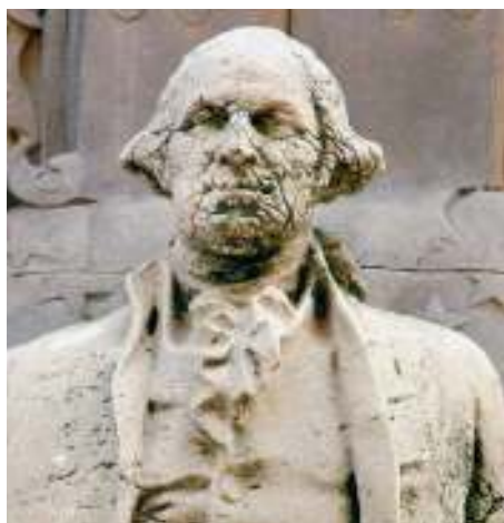
▲ A marble statue is being slowly dissolved by reaction of calcium carbonate with acid rain.
