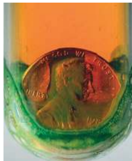
▲ Copper metal reacts with nitric acid ( \text{HNO}_3 ) to yield the brown gas \text{NO}_2 .
