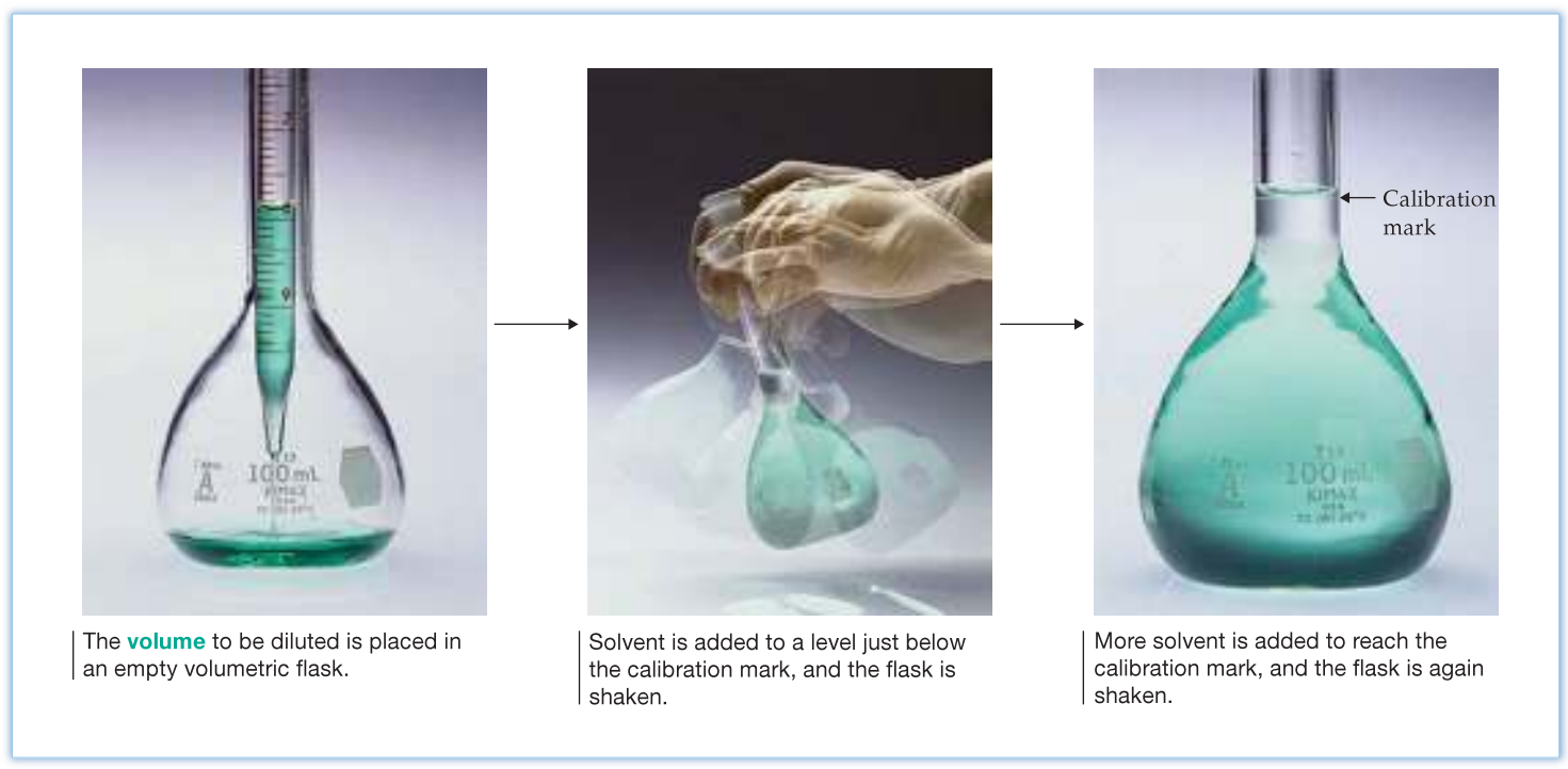
Figure 3.3 The procedure for diluting a concentrated solution.
