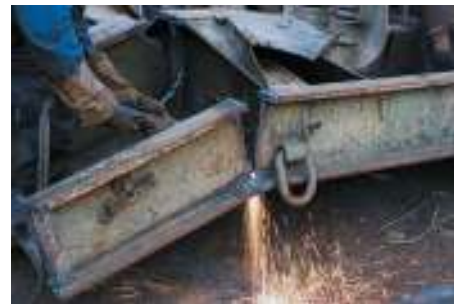
▲ Acetylene burns at a high temperature, making the reaction useful for cutting and welding iron.
