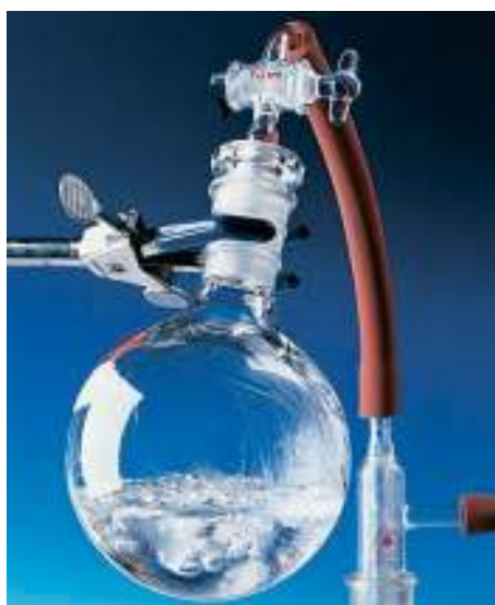
▲ At the triple point, solid exists in the boiling liquid. That is, solid, liquid, and gas coexist in equilibrium.
