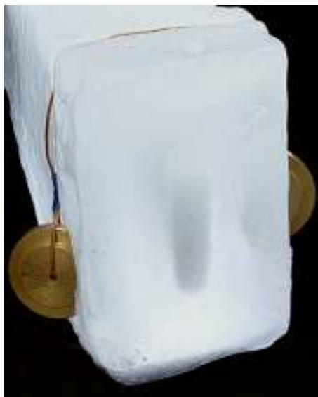
Figure 10.30 Pressure and melting point. Why does the weighted wire cut through this block of ice?
