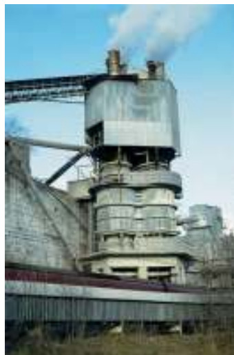
▲ The manufacture of cement begins with the thermal decomposition of limestone, \text{CaCO}_3 , in large kilns.
