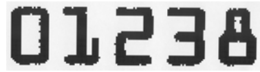
Figure 12.26: Some scanned digits typically used in optical character recognition. They were scanned into a computer which accounts for the obvious errors.
